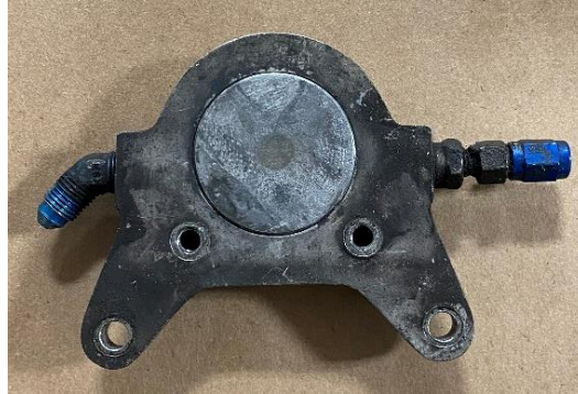
Figure 2, Original Matco Caliper, one 1.5" piston
