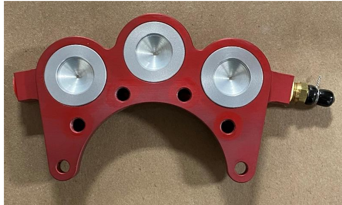
Figure 4, Three-piston Caliper Body, three 1.25" pistons
