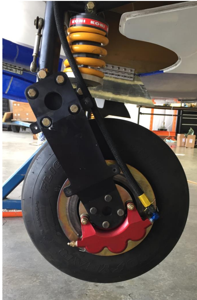
Figure 1, New Brakes Installed
