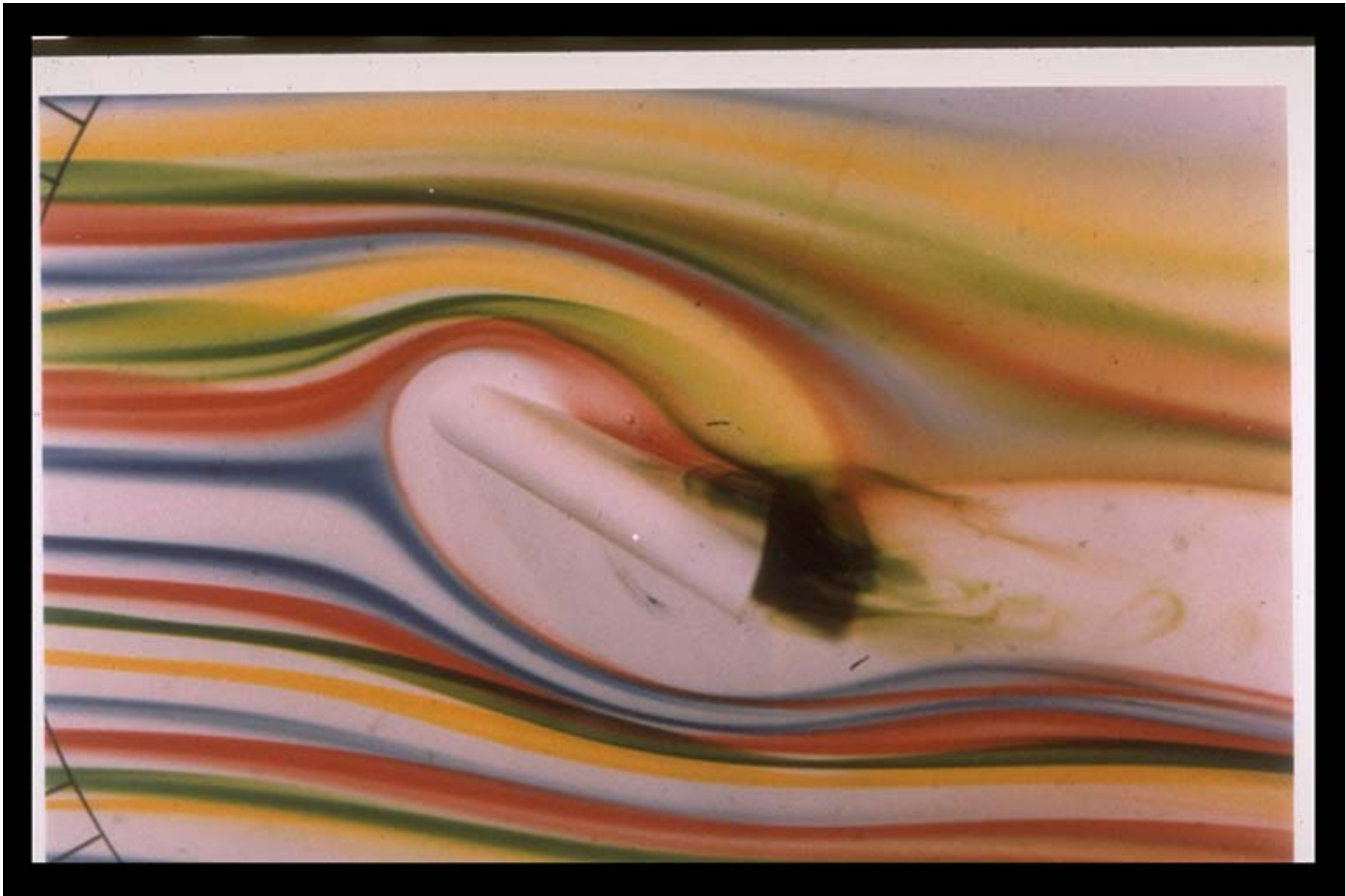
Water tunnel flow visualization by wall dye streaks. Triangular fin mounted on a flat plate. Flow from left.
