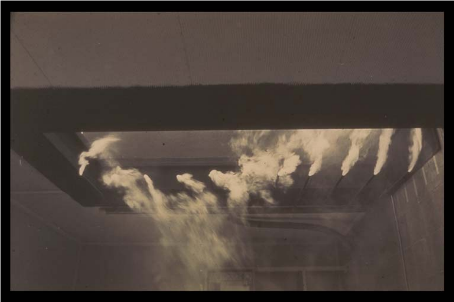
Smoke flow visualization in air. Reversed turbulent flow across an open door in a building.
