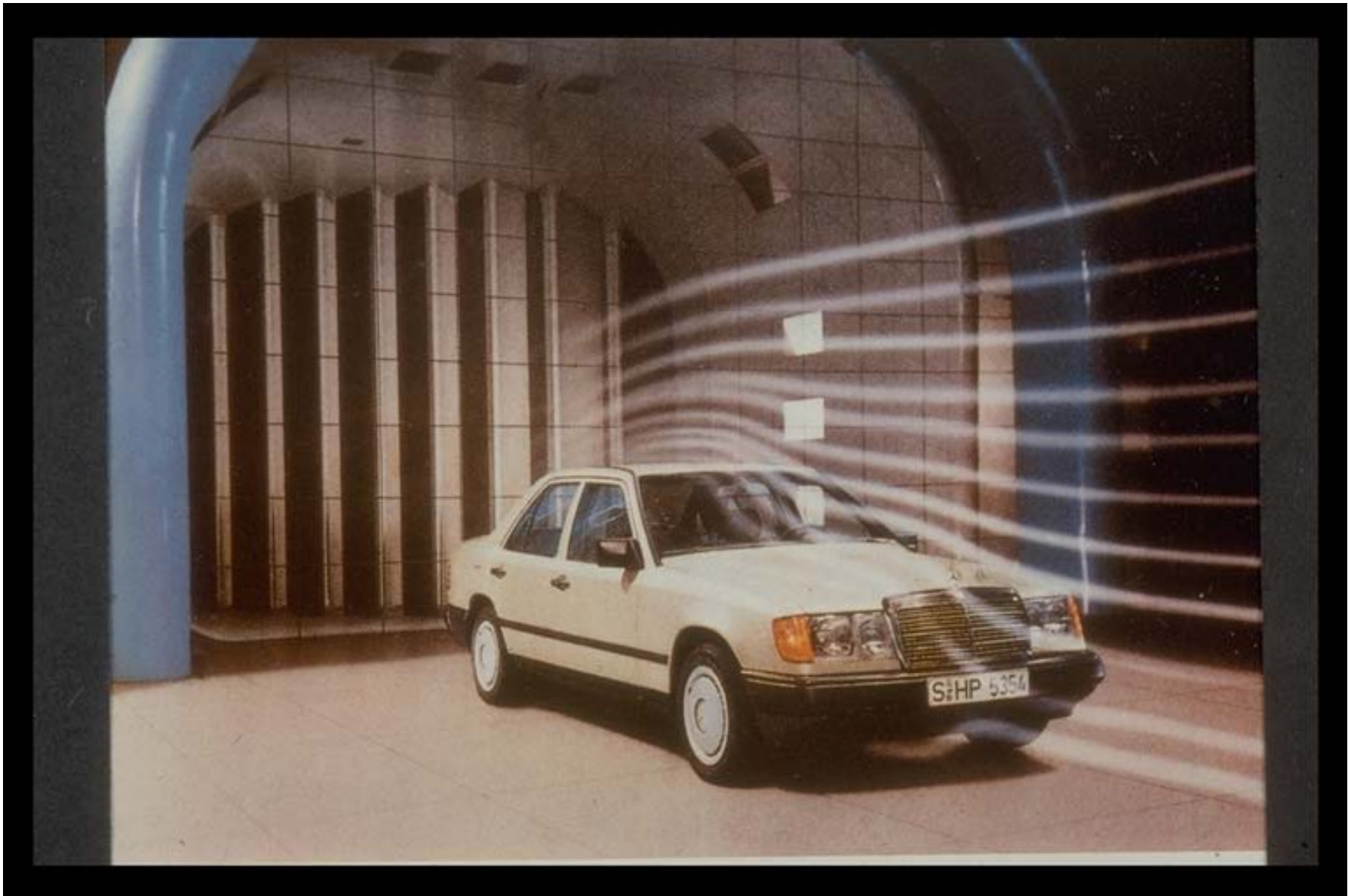
Smoke filaments flow visualization. (copyright not belonging to VKI)
