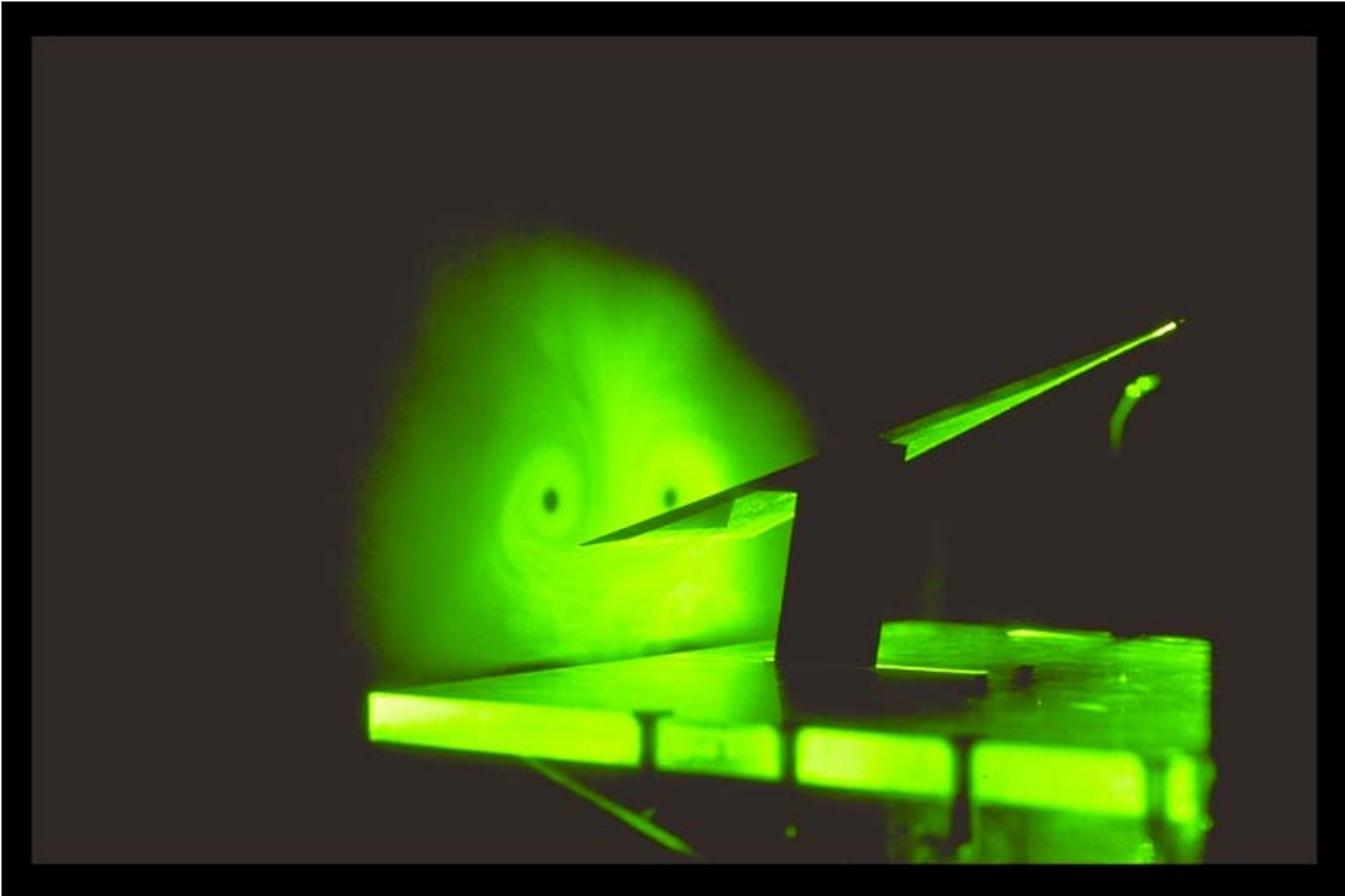
Smoke and laser sheet visualization of vortical flow on upper surface of delta wing.
