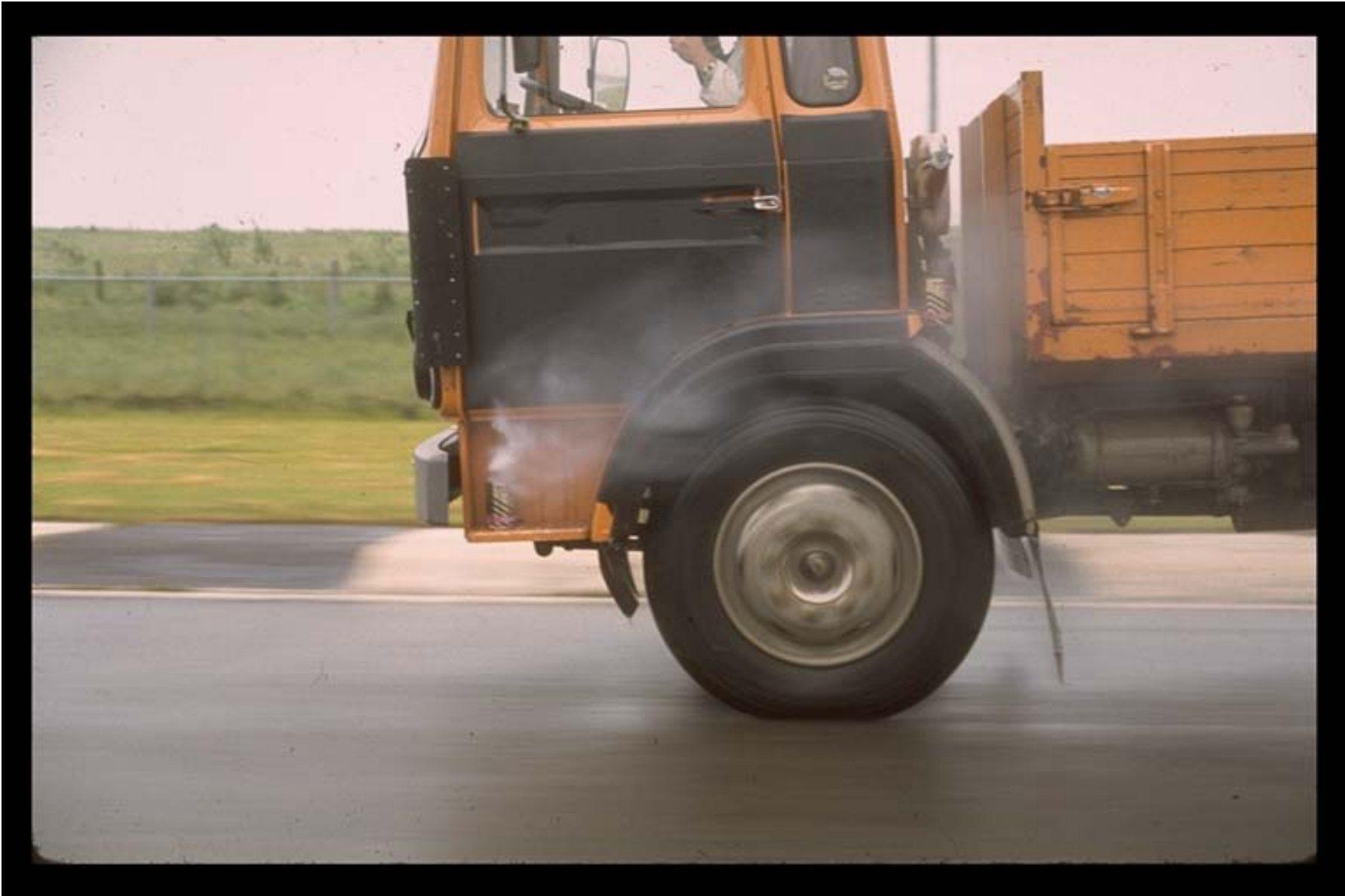
Smoke flow visualization of spoilers effectiveness in a truck to control flow separation on truck sides.
