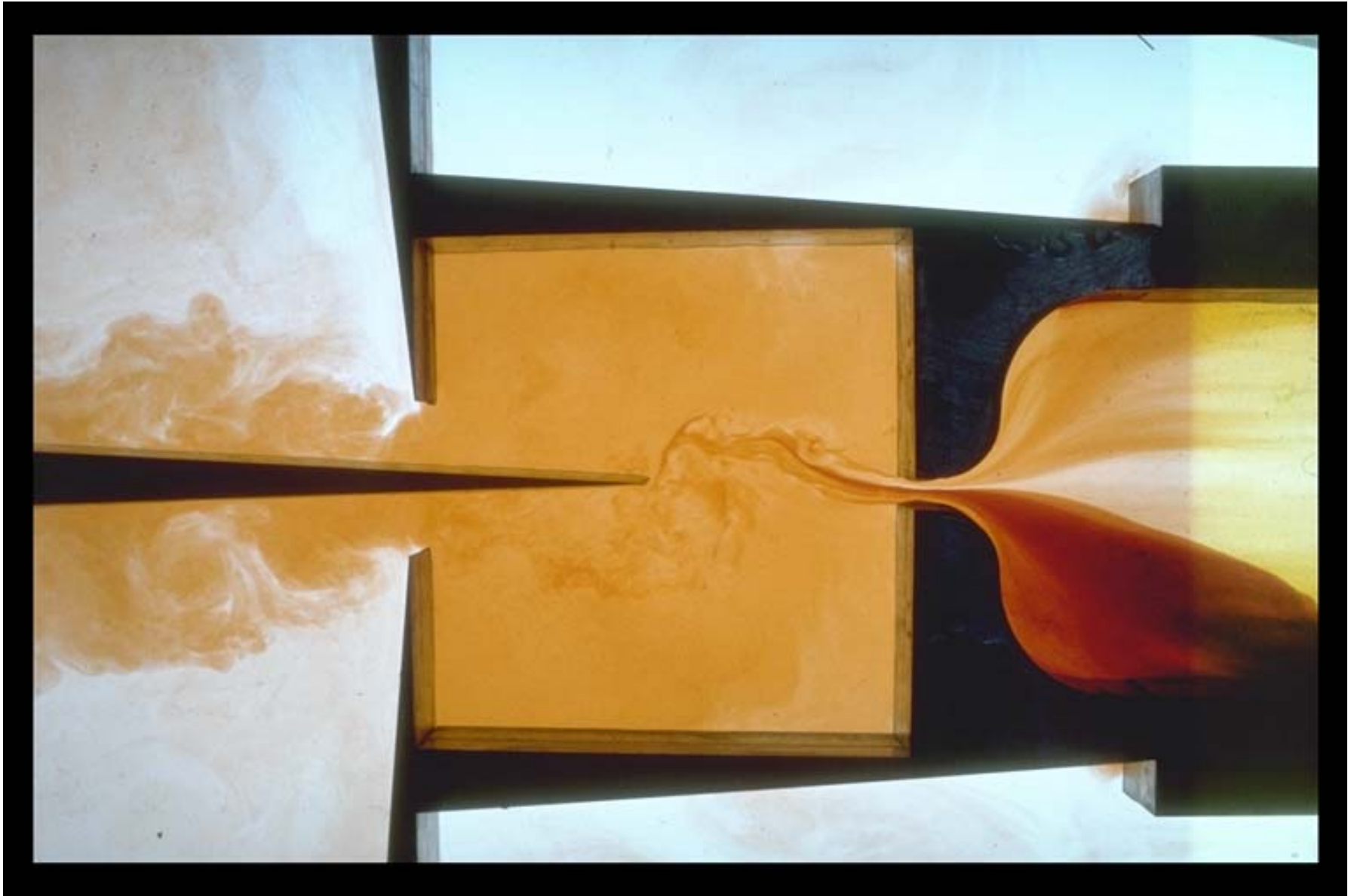
Colored water flow visualization: fluidic oscillator (jet-edge-cavity resonator) in a free-surface water table.
