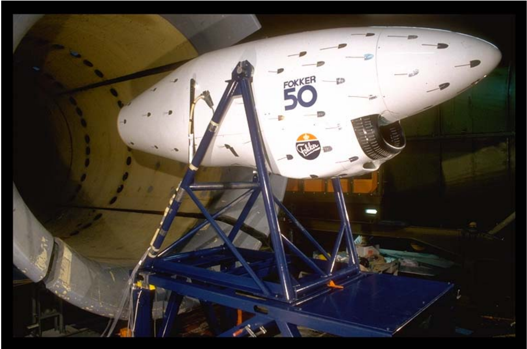
Wall tufts technique. Surface flow on a turboprop aircraft engine pod.
