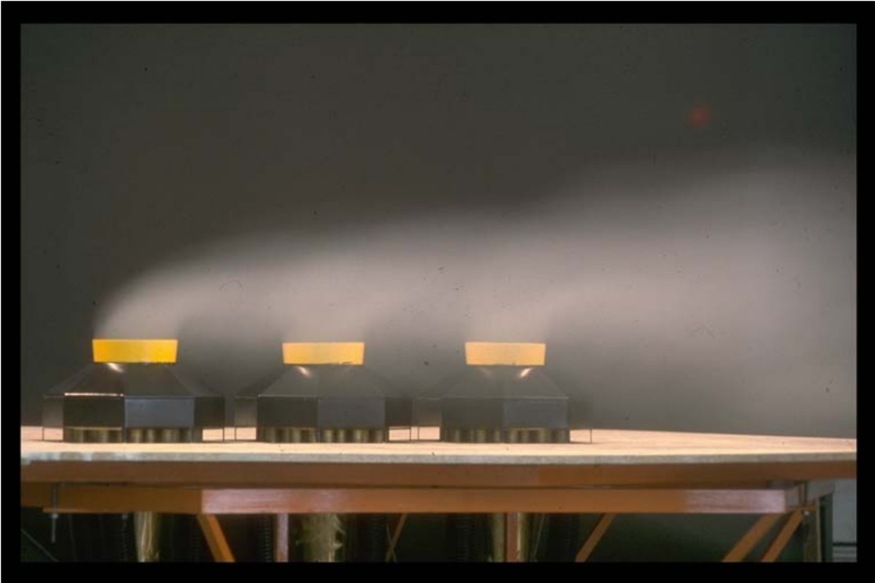
Smoke flow visualization of exhaust plume from forced draft cooling towers.
