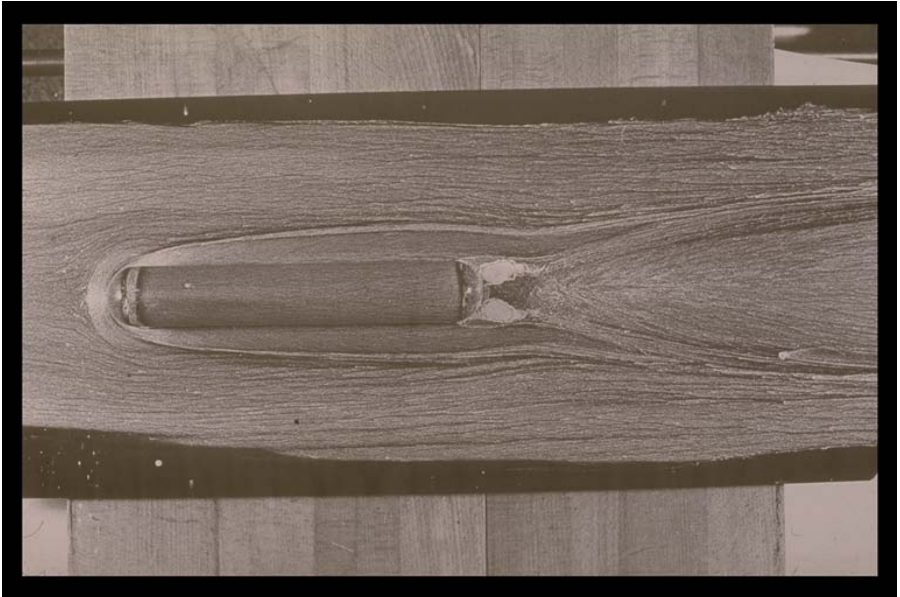
Oil flow visualization. Airflow around a bluff protuberance mounted on a flat plate. (top view, flow from left)
