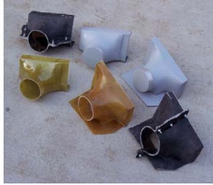
Diffuser plugs, mold and finished parts
