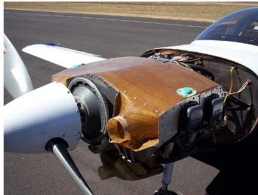
Diffuser and plenum chamber
