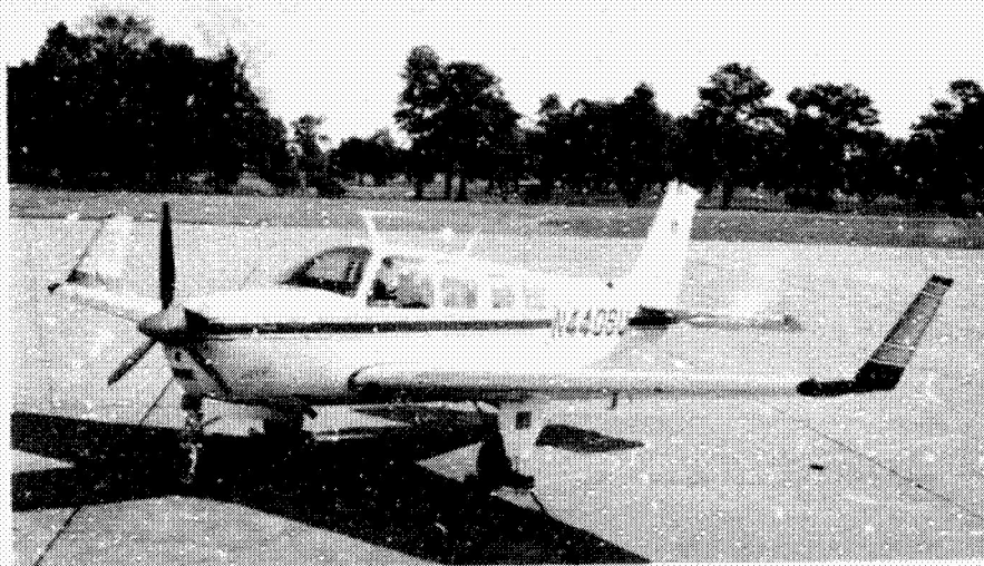
Figure 2.- Test airplane with winglets.
