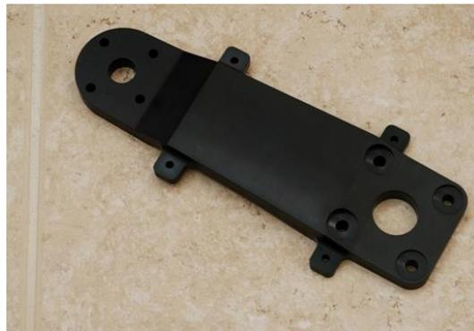
Figure 4, New Trailing with Gear Door Attachments
